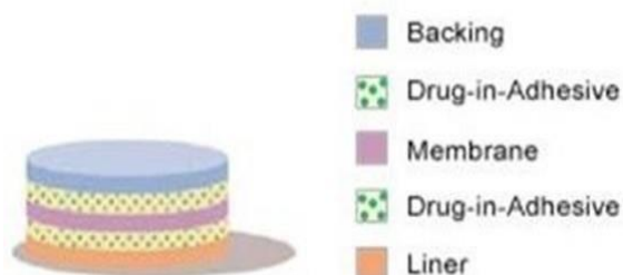
Figure 3: Multi-layer drug in adhesive.
